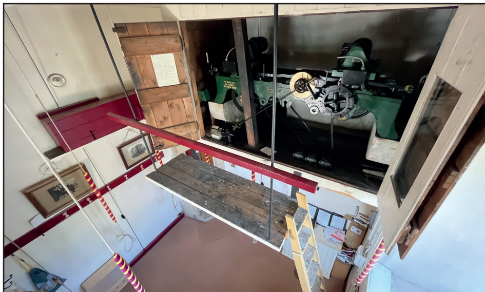
The clock mechanism is housed inside a large cabinet within the ringing chamber of the bell tower
